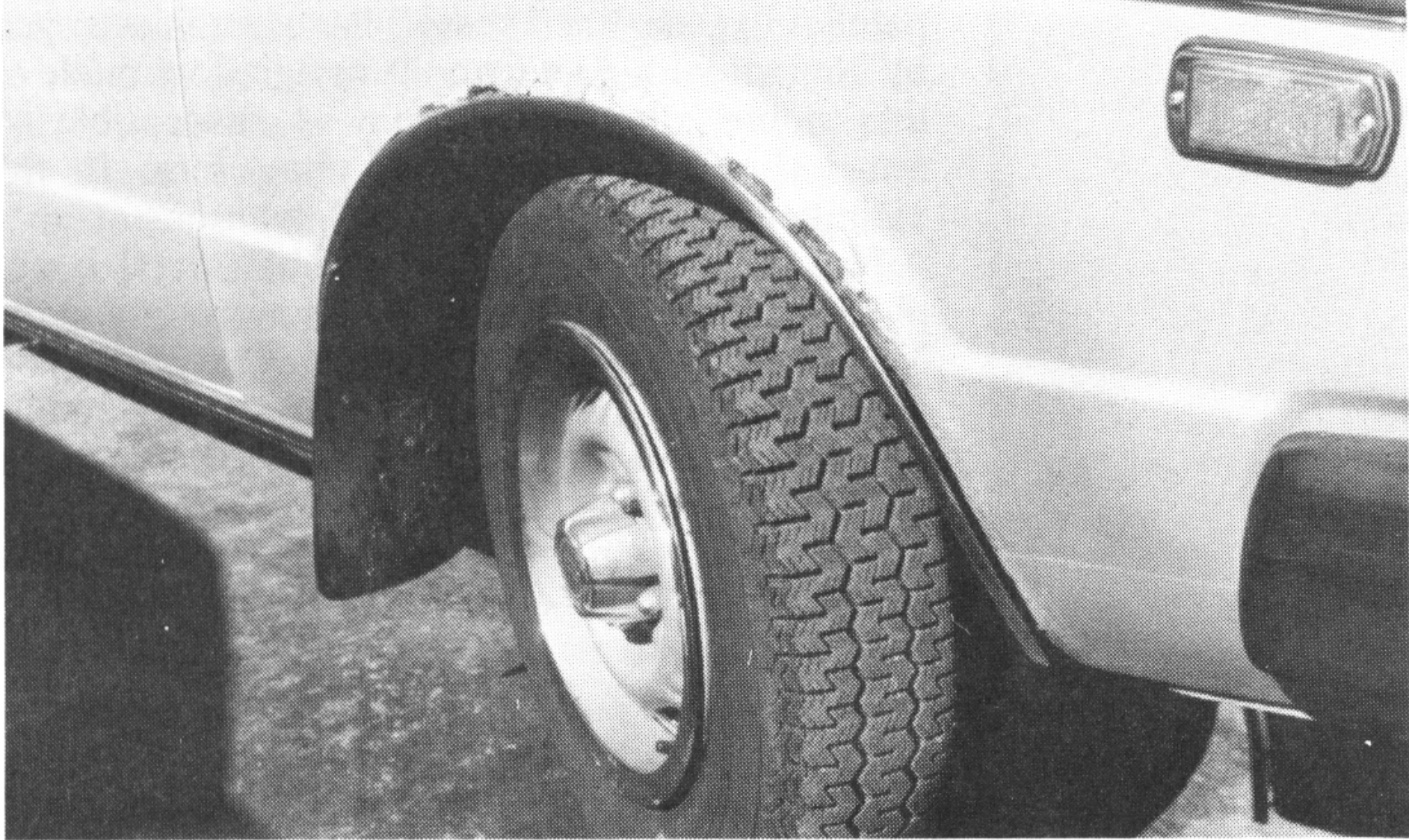
Galvanic corrosion of painted steel auto body panel in contact with stainless steel wheel opening molding.
