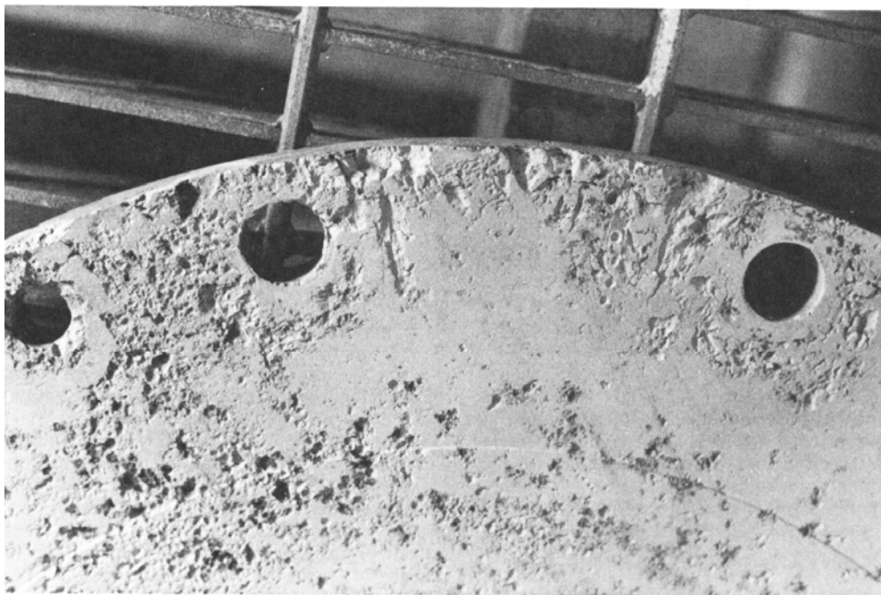
Two views of deep pits in a type 316 stainless steel centrifuge head due to exposure to \text{CaCl}_2 solution.
